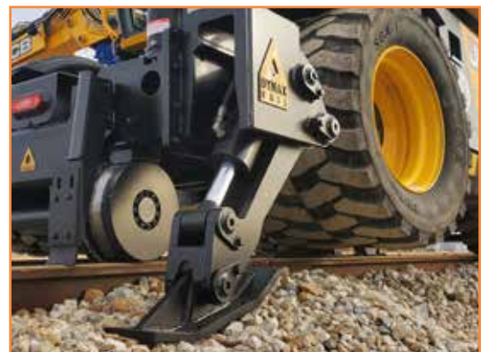
3rd rail stabilizers
