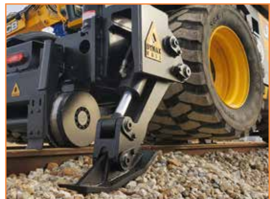
3rd rail stabilizers
