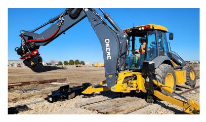
Backhoe Loader Cribbing Buckets are available with several tooth kits depending on your requirement. Models are provided with pins for attaching to common pin grab coupler systems. High strength construction and durability.
