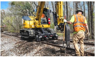
DymaxRail Cribbing Buckets for excavator machines are 8 inches wide but feature a longer tip radius, more capacity, and tougher construction to withstand higher forces. Shown here with optional thumb.
