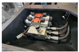
**Integrated Technology**Proportional control of multiple functions using factory auxiliary hydraulics.
