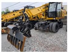
**Toolbar Attachment** Shown with ballast clearing blade installed
