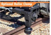
The optional roller clamp enhances safety in bridge work and overside applications by providing added stability where it's needed most.
