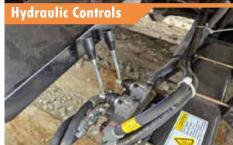
The hydraulic control group includes a 2 section manual valve to operate the front railgear and rear lift group, raising and lowering the rail wheels into position using the machine's existing hydraulics.
