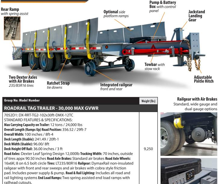
**OPTIONS:** Side platform ramps, insulated railgear, special track gauge, custom design solutions Design and specifications are subject to change without notice.
