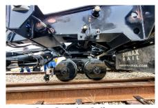
**Rear Rotating Railgear**DymaxRail innovative design for fast track access.
