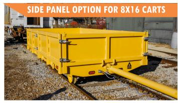
**7296D1-20T** 8ftx16ft with slip on 2 bin box. Features optional ratchet tie downs with straps.
