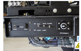
Control Panel Main power switches
