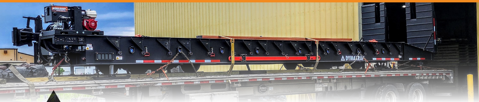
Hydraulic Ramps with rail pocket Heavy duty ramps with grouser grab bars
