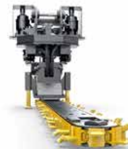
BALLAST BLASTER UNDERCUTTERS
